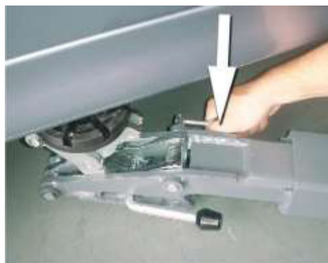
Figure 3: To release the fixture plate, the rear lever must be pushed.
