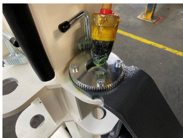
Grease upper aperture
