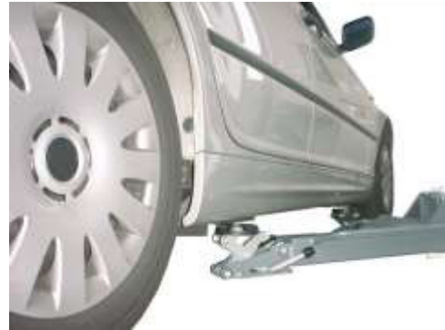
Figure 1: Position carrier plate below the fixture points approved by the vehicle manufacturer
