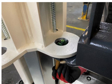
Grease the lower aperture
