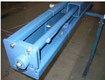
pic 4: fastened column elongation pieces
